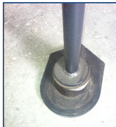
Profiled to suit curved edges around potholes.
