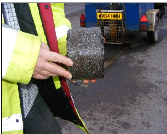
Viatec core – taken just 24 hours following compaction
